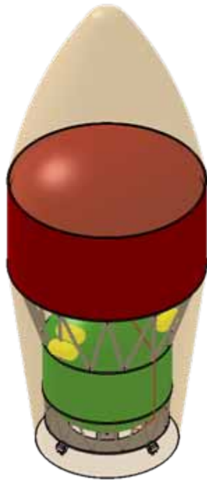
Tank Set in Launch Configuration
