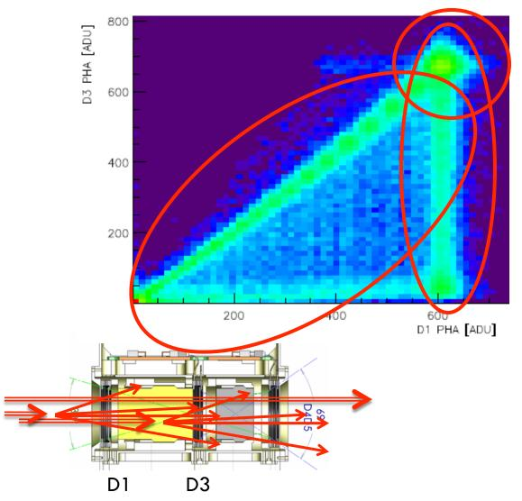
An iron enters the instrument and passes through it
