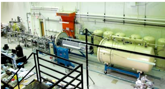
Figure 1. The 3 MV dust accelerator installed in the CCLDAS Lunar Environment and Impact Laboratory. The accelerator is used to simulate the effects of dust impacts with speeds \gg 10 km/s for micron sized projectiles. The facility will be also used to test and calibrate plasma and dust instruments, including the Lunar Dust Experiment (LDEX) for the LADEE mission. The facility is now operational and available for the lunar community for impact studies.
