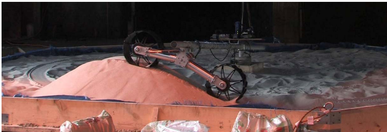
Drive mechanisms and wheel designs have completed several kilometers of terrestrial testing in lunar stimulant, using a counterweighted arm to mimic one-sixth gravity.
