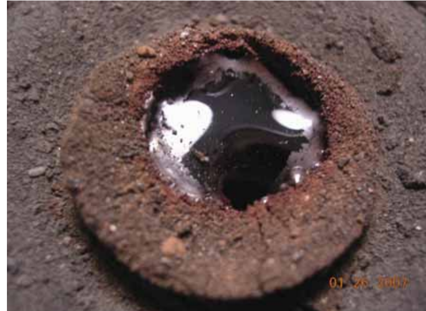
Vitrified JSC-1 Melt (dia. = 14mm; depth = 6mm)
