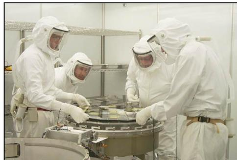
Fig. 1. Engineers, enclosed in HEPA-filtered suits, assemble Genesis collectors into the science canister inside of an ISO Class 4 cleanroom at Johnson Space Center. Small pieces of cleaned aluminum foil are used to grasp the collector array, so that gloves never directly touch the hardware.
