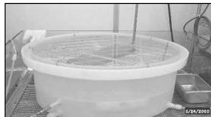
Fig. 2. Genesis array frame is cleaned with flowing UPW in a 30-inch diameter cascade tank enhanced with ultrasonic energy.
