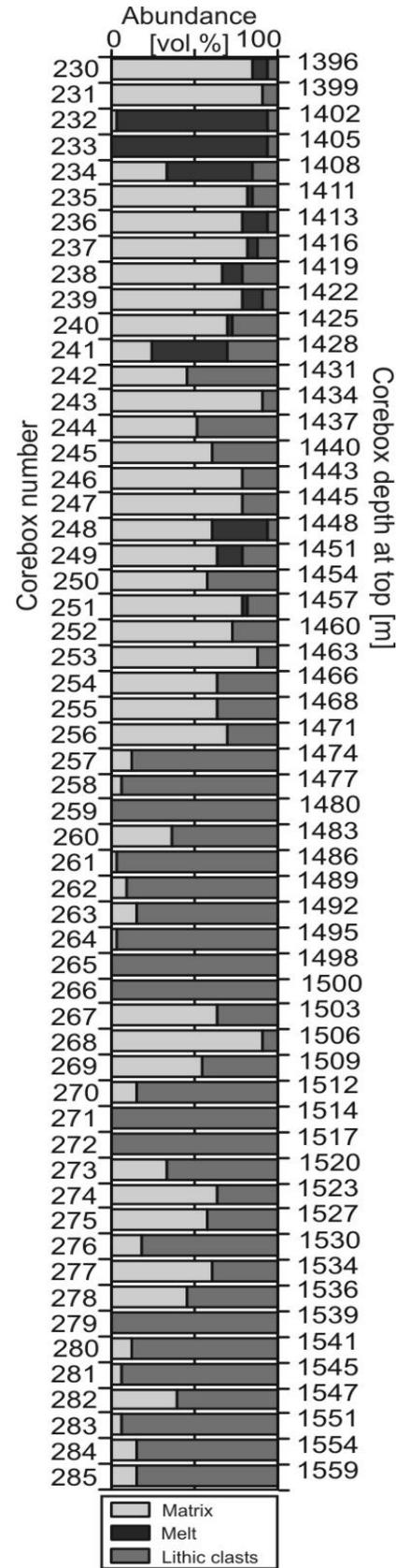
Fig. 1 Melt pods and lithic clasts >4,8 cm in impact breccia section of drill core Eyreville-B.
