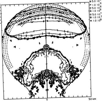
Figure 2. Pressure Contours for a 5 km/sec Impact of a 10 km into a 100 km Silicate Asteroid
