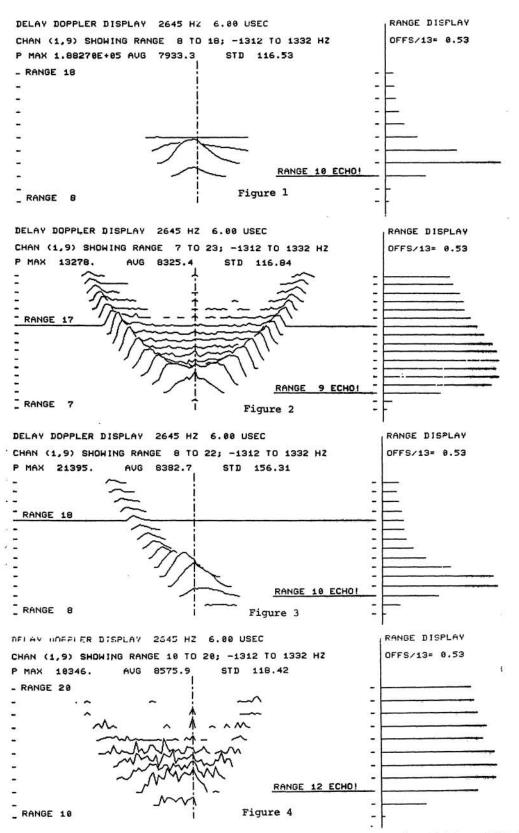
Delay-Doppler radar echoes observed on 14 December 1990. UT times are: 06:01:52, 06:22:10, 06:42:28 and 07:21:27 respectively corresponding to Longitudes 109, 114, 119 and 128.
