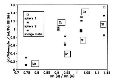
Fig. 1 Correlation of element depletions with boiling point for 2 ~10 micron metal spheres and "sponge" metal from the 40.3 GPa target.
