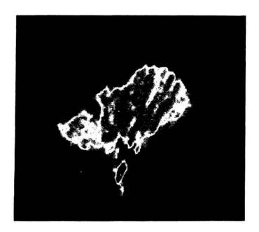
Figure 1: Scanning Transmission Ion Microscope (STIM) image of the density distribution through the interior of a 40  $\mu m$  fragment of Allende matrix.
