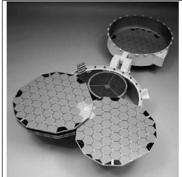
Fig. 1. Model of the two Genesis solar-wind collectors. First, the four deployable passive collector arrays (comprised of individual hexagon collectors; here, only dummy-materials shown). Second, the electromagnetic concentrator (round, inside canister of spacecraft). The collector arrays can be rotated to fit inside a canister, the base of which is in partial view next to the concentrator A 5<sup>th</sup> collector array is in the canister cover(upper right corner of the photo).
