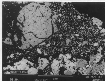
Photograph 1. A backscattered electron image of the brecciated part of the impact rock from the Ramsö island.
