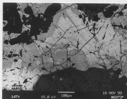
Photograph 2. A backscattered electron image of radial potash feldspars with glass rim towards the quartz (Q) aggregates.
