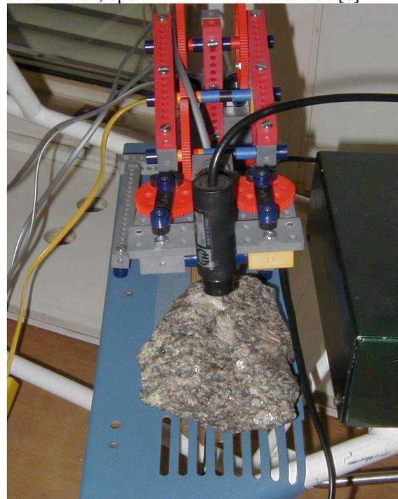
Fig. 2. The rock radiation measuring assemblage.
