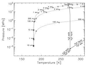
Figure 2: Example geothermal profiles, for ice-cemented soil (top curve), weakly cemented sandstone (middle) and loose, dry soil (bottom curve).
