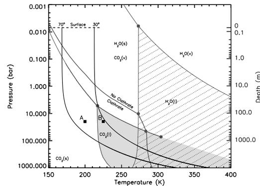
Figure 1: H<sub>2</sub>O-CO<sub>2</sub> equilibrium phase diagram with Martian geotherms at 30 and 70° latitude, the observed latitude range of the gullies. Geotherms assume an internal heat flux of 30 mW m<sup>-2</sup> and thermal conductivity at the surface of 0.3 Wm<sup>-1</sup>K<sup>-1</sup> exponentially increasing to 3.0 Wm<sup>-1</sup>K<sup>-1</sup> at depth. Regolith structure assumes 20% surface porosity with decay constant 2820 m (Clifford 1993). The surface pressure is 7 mbar.
