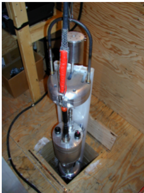
Fig. 1. Plastic 0.3 by 1.2 m collector body (white) containing filter fabric. Spiked wheels (top one visible) provide mobility; stainless steel central waterproof housing contains motors and pump.
