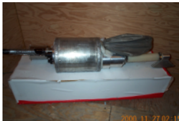
Fig. 2. Modified collector. Particles are suctioned by axe-shaped nozzle (right), go through the pump and into filter bag. The spiked wheels are not visible.
