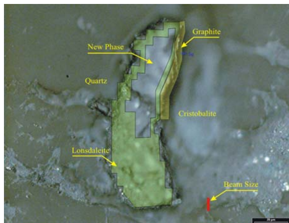
Figure 1.: Fine scale textural relations of the new polymorph of carbon (colored blue), lonsdaleite (colored green) and secondary graphite (colored brown) as obtained from Synchrotron micro-beam x-ray diffraction and fluorescence mapping studies. The length of black scale bar on the lower right corner is 20\mu\text{m} .
