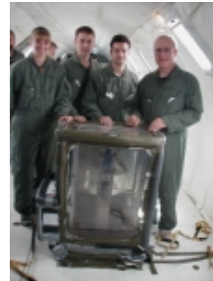
Fig. 2. The collector test fixture aboard the KC-135 microgravity test facility, with experimenters Melissa Franzen (University of Arkansas), Paul Bartlett (Honeybee Robotics), John DiPalma and Jeff Preble (SpaceWorks, Inc).
