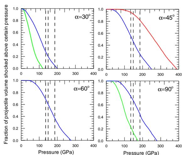
**Fig.1.** Maximum shock pressure distribution in the projectile for different impact angle  $\alpha$ . Green lines show results for  $V=15$  km/s, blue lines show results for  $V=20$  km/s, red line shows results for the impact on dunite target. Dashed vertical lines indicate incipient melting pressure 135 GPa, complete melting pressure 149 GPa, and incipient vaporization pressure 186 GPa for dunite [9].
