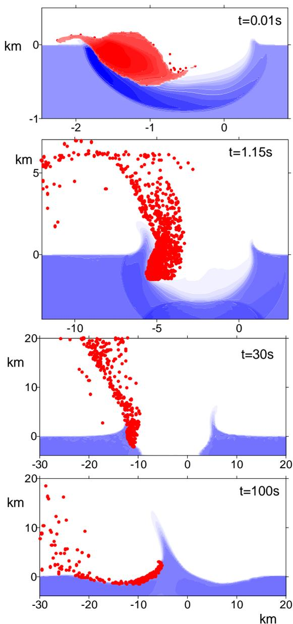
**Fig.2.** Distributions of water and impactor material after the oblique 45° impact of a 1-km-diameter projectile at 20 km/s. Impactor material is shown by red.
