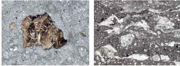
Fig. 2: Brown fluorite – silicate clasts in fine grained dolomite dike groundmass. Sample YAX-1_1314,77 m, thin section, plane polarized light, width 2.25 mm. Fig. 3: Light grey streaks of anhydrite and rounded clasts of dolomite in a fine grained dolomite dike groundmass. Sample YAX-1_1373,95 m, thin section, plane polarized light, width 1.8 mm.
