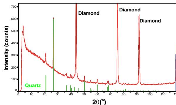
Figure 2: X-ray diffraction pattern of quartz powder in a CVD diamond core. Diamond reflections are marked, and a standard pattern for quartz (ICDD card #33-1161) is superimposed.
