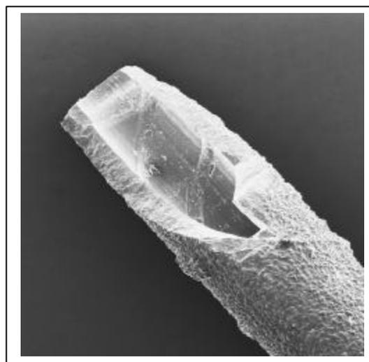
Figure 1: Secondary-electron image of a spiral CVD diamond core, broken open to show spiral grooves. Drill-core wall thickness is 150  $\mu\text{m}$ .
