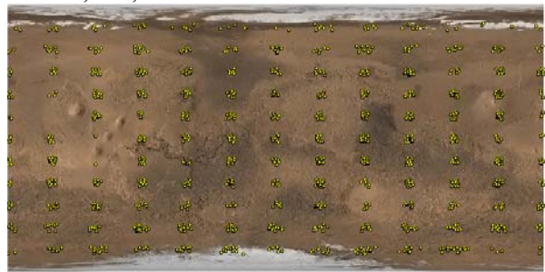
Figure 1: 1,216 MOLA (tie) control points, measured in groups with a spacing of 30° in longitude and 15° in latitude (the background is a MOC Mars mosaic, with 0° longitude at center and east to the right).
