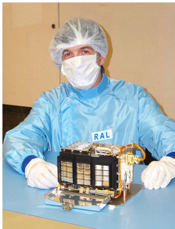
Figure 1: The D-CIXS instrument, fully assembled. Note the three facets each with 8 swept charge devices. The door protects the instrument from proton damage. The total mass of D-CIXS is ~4.5kg
