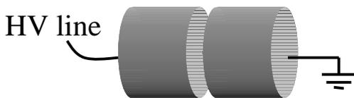
**Figure 1.** Schematic showing the parallel-plate geometry of the brass electrodes. High voltage was applied using both polarities.
