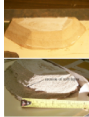
Figure 1: Sandstone simulant prior (left) and after (right) abrasion.
