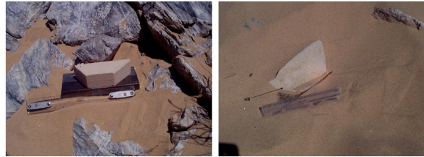
Figure 4: Before and after pictures of sandstone simulant target of same composition as targets used in wind tunnel experiments. Sill formation seen on this example. New pits were found in other targets. Target lost 60% of its mass during its 6 months of exposure.
