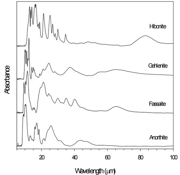
**Figure 2.** Far-IR spectra from candidate circumstellar grain types. Anorthite (Lake Co. OR), fassaite (Val di Fassa, Italy), gehlenite (Allende meteorite), and synthetic hibonite. Anorthite and fassaite are common minor phases in primitive IDPs.
