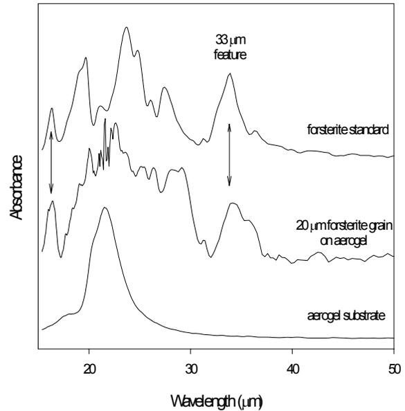
**Figure 3.** Far-IR spectra of the forsterite standard, the aerogel substrate, and a single 20  $\mu\text{m}$  forsterite grain on an aerogel substrate.
