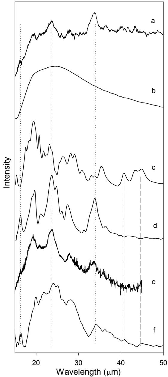
**Figure 1.** Far-IR spectra for amorphous olivine (b), clinoenstatite (c), forsterite (d) and IDP L2005\*A4 (f). Also shown are ISO spectra from HD100546 a young stellar object [5] (a) and comet Hale-Bopp [4] (e). Dashed lines and dotted lines indicate prominent clinoenstatite and forsterite bands, respectively.
