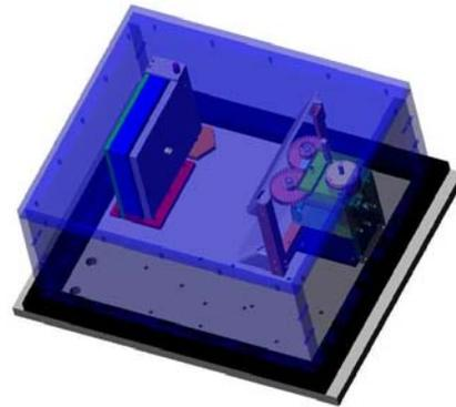
**Figure 1.** Schematic of a PRIME Impact Chamber. The target material is held in place in the target chamber at left until the airplane is in a stable low-acceleration part of the parabola. The target surface is exposed by manually opening a door through a mechanical feedthrough. The projectile launcher is shown configured for a normal incidence impact at right.
