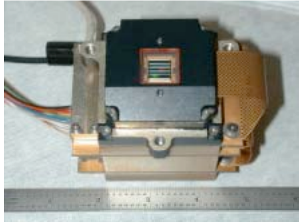
Figure 1. The Odyssey THEMIS VIS instrument. The color filters can be seen overlying the CCD at center.
