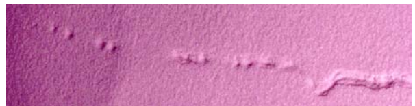
Fig. 2. Image showing slightly irregular trace of model pit chain. Trough at right consists of intersecting pits. Illumination from lower right. Image width is approximately 18 cm.
