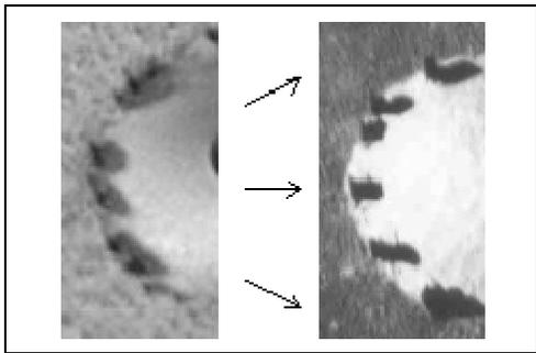
Fig. 1: Using the data from image MOC2-323, a model (right) was created and photographed with the same camera and light source angles. The resulting shadows in the model are a close match to the gray spots in the MOC2-323 image (left).
