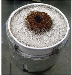
Samples were frozen at -85°C overnight. Once thoroughly frozen, simulant mixtures were drilled on a mill using a 1.4 cm diameter wood auger composed of stainless steel and connected to a 360° rotational torque sensor. The sample was drilled at a rate of 500 revolutions/min with a decent rate of 6.45 centimeters/min. The final drill depth was 11.3 centimeters.
