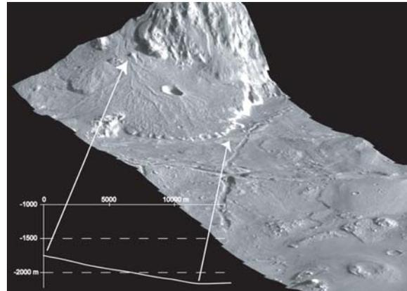
Fig. 4 - 3D representation of an alluvial fan. (THEMIS V03210003 image draped on MOLA data)
