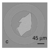
The absorption CT sections show a network of fractures in the studied grain and a few [m-thick layer formed on the grain (Figure c). The 3D facet orientation allows identifying the crystalline phase (olivine) of the studied grain; the X-ray attenuation coefficient permit to estimate its average composition
