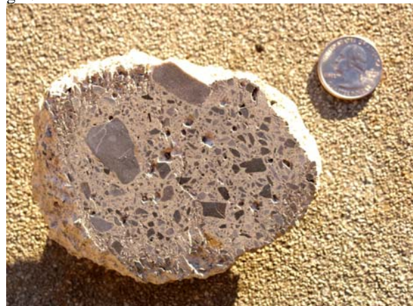
Fig. 2: Section of breccia sample collected in the Howell structure showing angular clasts welded in a fine grained friable matrix.
