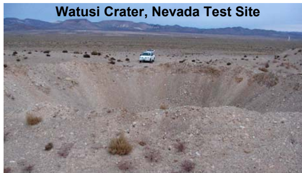
Fig. 1: Watusi , a high-explosives experiment in alluvium by Los Alamos National Laboratory scientists, September 2002. It is ~24 m diameter. Small craters expose near-surface material for identification via infrared remote sensing, both terrestrially and on Mars.
