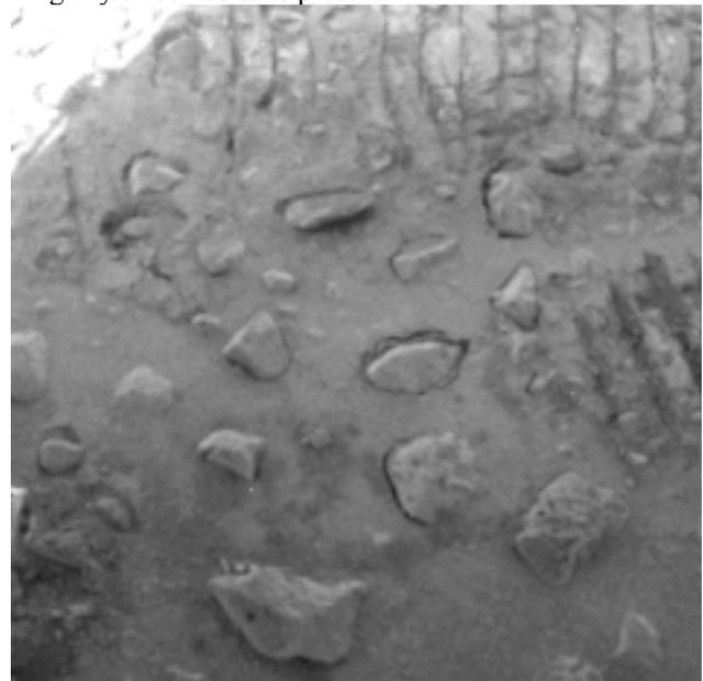
Figure 1: a view of the track of the Spirit rover, showing small rocks pressed through the crust layer by the rover wheel.
