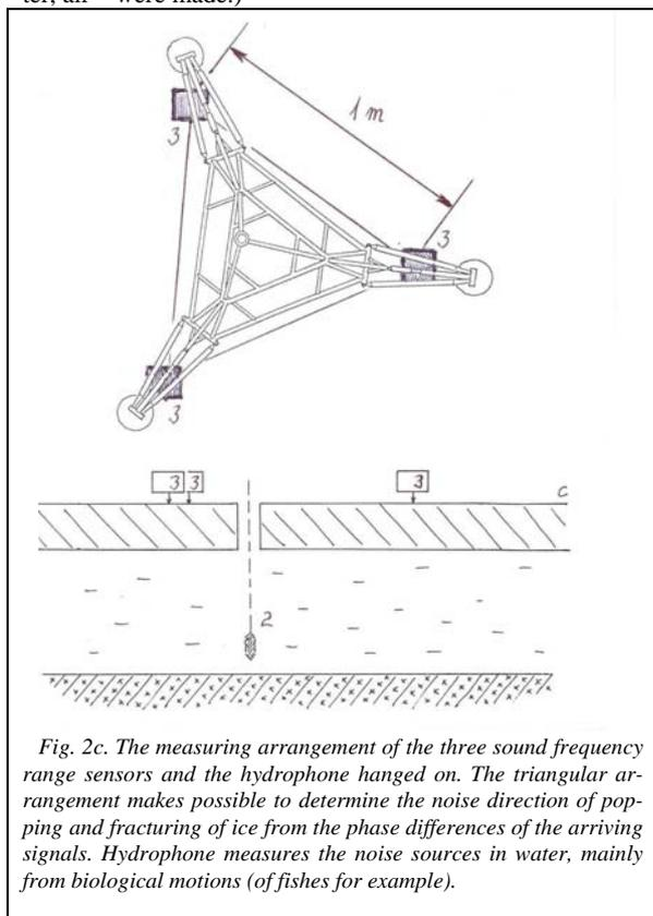
Fig. 2c. The measuring arrangement of the three sound frequency range sensors and the hydrophone hanged on. The triangular arrangement makes possible to determine the noise direction of popping and fracturing of ice from the phase differences of the arriving signals. Hydrophone measures the noise sources in water, mainly from biological motions (of fishes for example).
