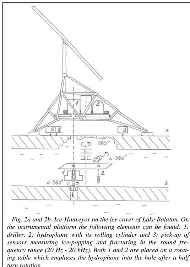
Fig. 2a and 2b. Ice-Hunveyor on the ice cover of Lake Balaton. On the instrumental platform the following elements can be found: 1: driller, 2: hydrophone with its rolling cylinder and 3: pick-up of sensors measuring ice-popping and fracturing in the sound frequency range (20 Hz - 20 kHz). Both 1 and 2 are placed on a rotating table which replaces the hydrophone into the hole after a half turn rotation.
