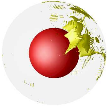
Figure 3: Temperature- and depth-dependent viscosity mantle. Ra=2*10^7 , E=157 kJ/mol, V=6 cm 3 /mol, H_{int}=1.54*10^{-12} W/kg. The upper mantle viscosity has been reduced by a factor of 50. Degree-1 forms very quickly.
