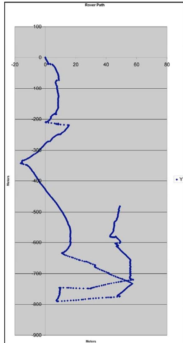
**Fig. 2.** 1.3 km traverse of SR2 during the 2002 Anza Borrego field test. This traverse was executed in a single afternoon, at an average speed of ~400 m/hour.
