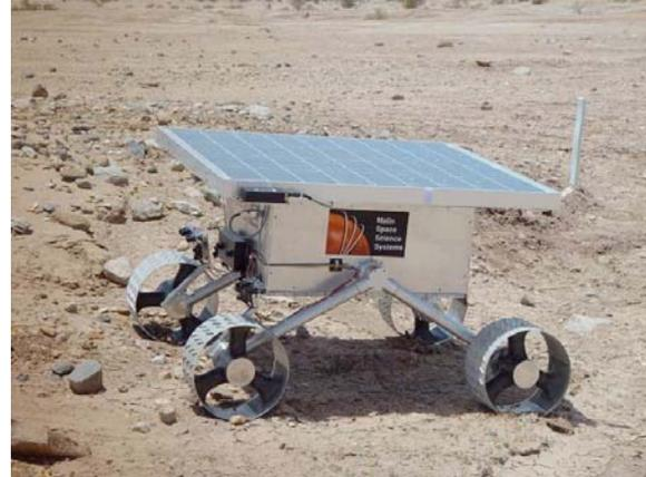
**Fig. 1.** The SR2 rover during the Anza Borrego field test in 2002. For scale, the vehicle's wheels are 20 cm in diameter.
