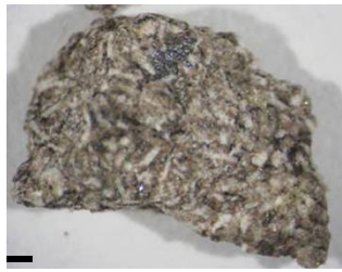
Fig. 3. Chip of LAP 02224 (31) used for bulk chemical analysis. Plagioclase and mafic mineral phases are visible. Scale bar is 1mm.
