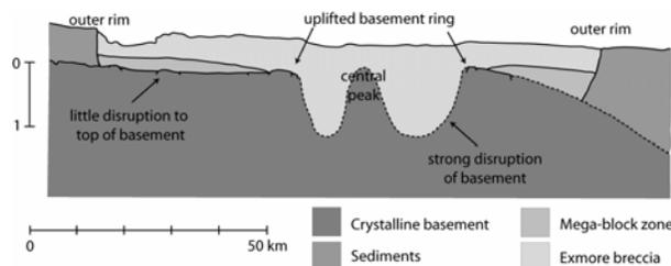
**Figure 1.** Schematic cross-section of Chesapeake Bay Impact Structure based on interpretation of seismic data and drill cores [2,7-10]. Dashed line indicates uncertainty in exact location of top surface of the crystalline basement.
