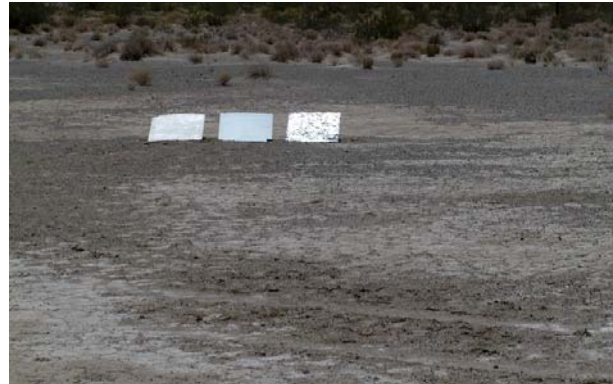
Figure 1: Bristol Lake Site. Gypsum bearing rock exposed as slightly brighter regions, darker regions are silty. Three aluminum targets used for downwelling radiance correction are approximately 1 x 1 meter [5].
