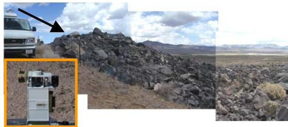
**Figure 4:** Danny Boy ejecta, south rim, looking ~east. RamVan is on the Danny Boy rim, on a dirt ramp constructed for crater access. The arrow marks an example view from the spectrometer (shown in inset) that is raised above the roof.
