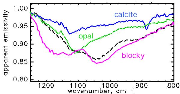
**Figure 5:** RamVan spectral data [8]. These spectra are from the Danny Boy southwest interior. The purple, solid trace is of blocky material. The green and blue traces match lab spectra of opal and calcite, respectively. The dashed, black trace illustrates additional spectral variety.
