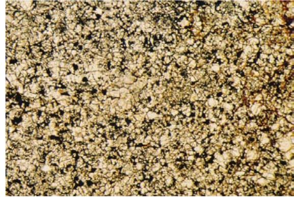
**Figure 1.** Plane-polarized light image of NWA 3100 showing the very fine grained, polygonal-granular texture (width of field = 5 mm).
