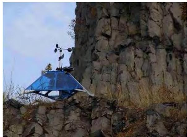
*Fig. 4. Hunveyor-4 studies columnar basalt flow environment at Hegyesztű, North-Balaton Mountains, Hungary.*
