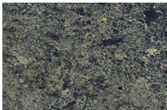
Figure 4. Cross-polarized thin section image, showing maskelynite (dark) and very fine grained olivine and pyroxene. Width of field = 8 mm.
