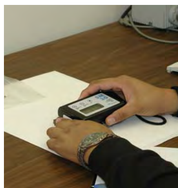
Fig. 1a. Sample of the “Chico” meteorite being measured on contact with SM-30 susceptibility meter over a wooden table.
