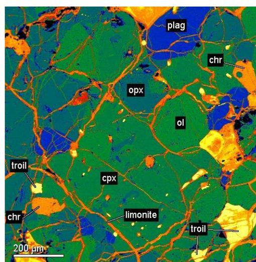
**Figure 2.** False-color, back-scattered electron image.
