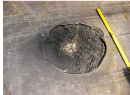
Fig. 3a Exp 2809, crater in wet sandstone block
